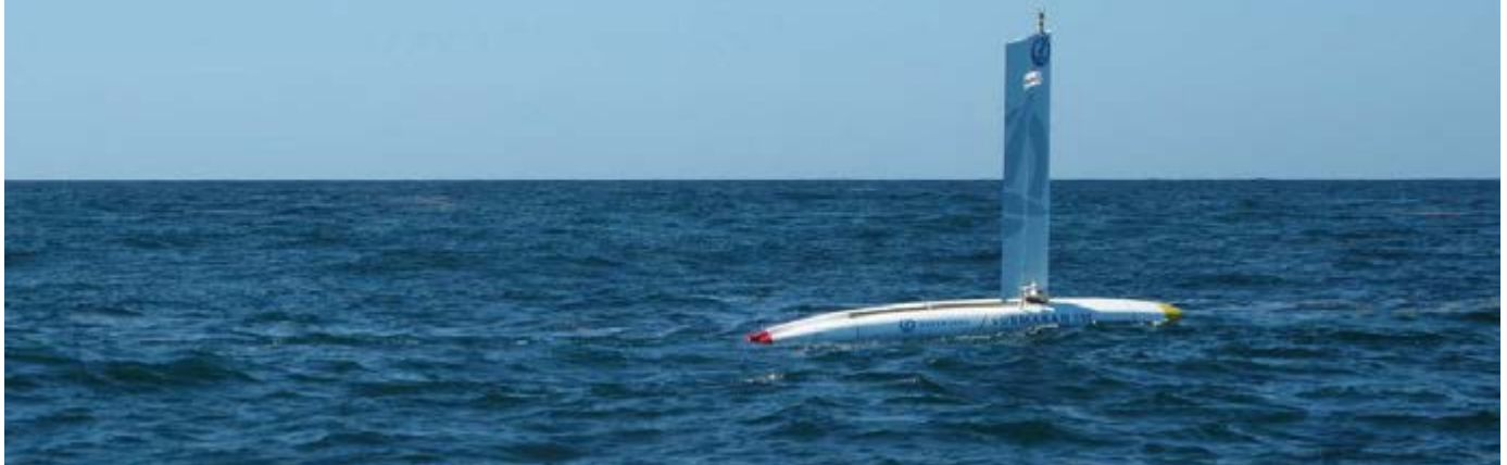
Ocean Aero's Submaran S10 uses composite materials for its unique sail. (Photo: Ocean Aero)
